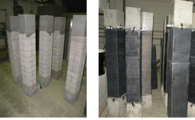
Figure 1. Reinforced masonry columns before (left) and after (right) FRP wrapping
