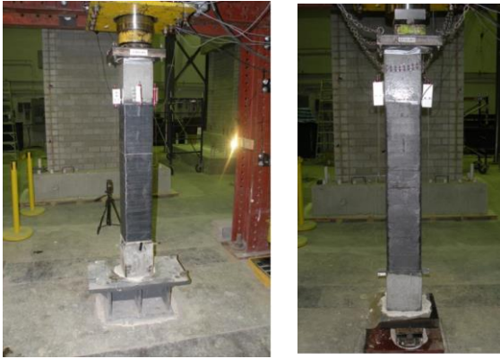
Figure 2. Testing of FRP-confined reinforced masonry columns under concentric and eccentric axial compression
