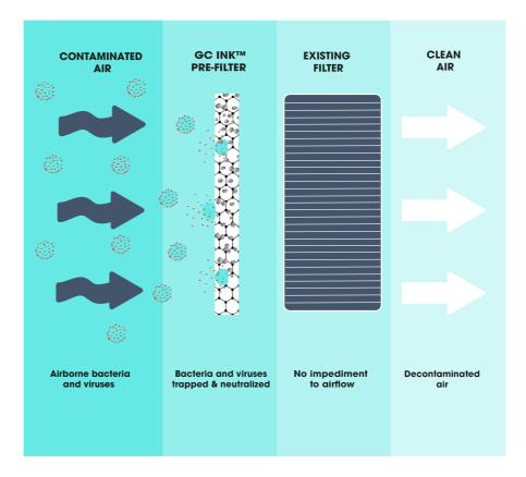
When used in filters and masks, GC Ink™ is highly effective at trapping and neutralizing airborne coronaviruses and other viruses/bacteria for several weeks.
