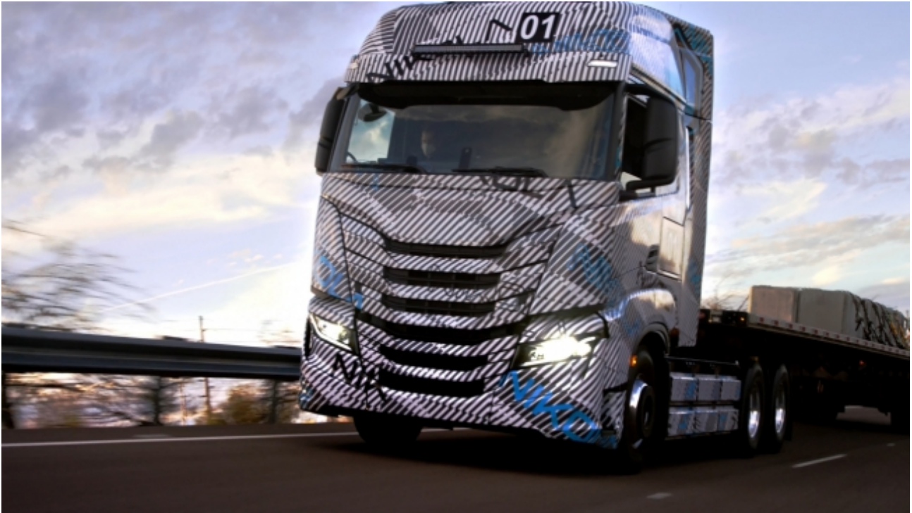
Nikola Tre battery-electric vehicle (BEV) prototype
