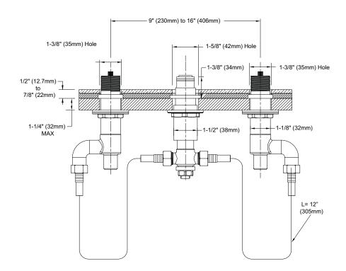
IMPORTANT NOTE: This valve/trim can only be installed in a built-up deck. It cannot be installed on pre-finished deck or on tub rim.
