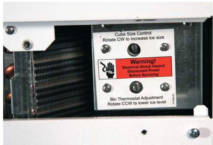
Condenser and Bin Thermostat
