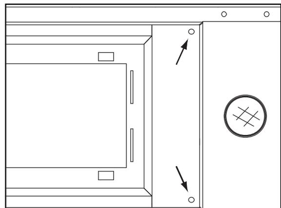
2. Secure filter bracket to AK8000AS body by installing a bracket screw into each of the (4) corners.
