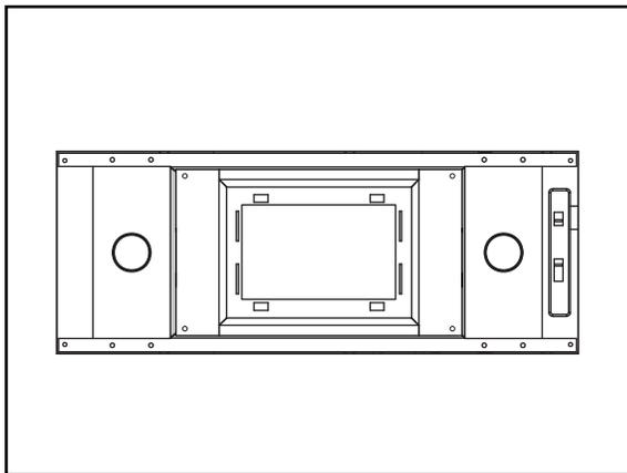
1. Position and install charcoal filter bracket into AK8000AS as shown above.
