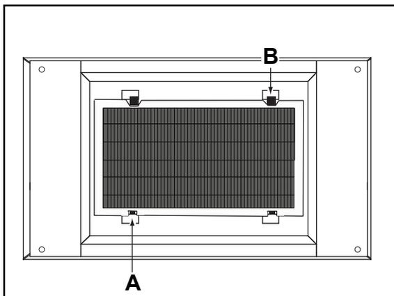
3. Install charcoal filter (plastic side up) into filter bracket. Insert tab cut-out side **A** of charcoal filter into bracket first. Lock charcoal filter into place by pushing down on side **B** with locking tabs.
