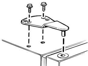
*Installing the hinge on the left.*
