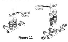
• Secure ground clamp to metal pipes.
