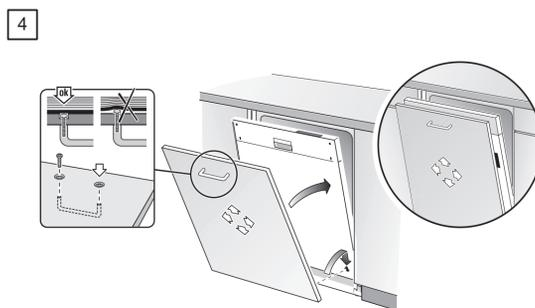
Insert metal mounting brackets at bottom of door. Then press the top of the door to attach to the dishwasher. Position door as necessary.
