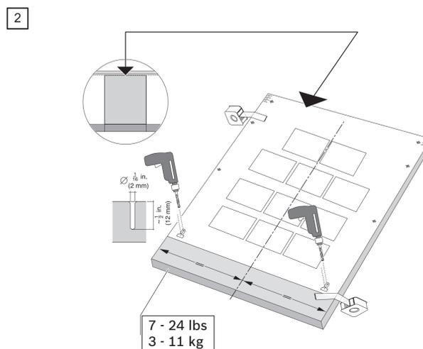
Before beginning the custom panel installation, make sure the dishwasher is fully installed according the installation instructions. The top of the unit should be a minimum of 6mm from the counter and centered in the space. Be certain that the panel being installed is completely flat with no warpage. The top of dishwasher should be flush or lower than the adjacent cabinets.\*
