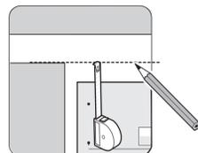
\* If the dishwasher will not raise to the height of the adjacent cabinets, measure the difference and move the template down on the custom panel by the same distance.
