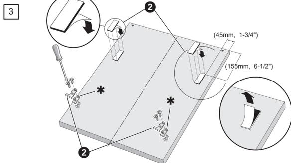
If your unit came with a rubber apron, you will need to use the plastic spacers during your custom panel installation. Place one plastic spacer between each metal bracket and the panel, if required. Attach the metal brackets 2 as shown. Install the hook and loop fastener strips, exposing adhesive on both sides of each strip.
