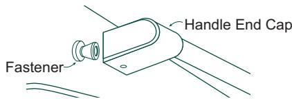
**NOTE:** When installing Statement horizontal handles, position the handle so that the set screws are facing downward.
