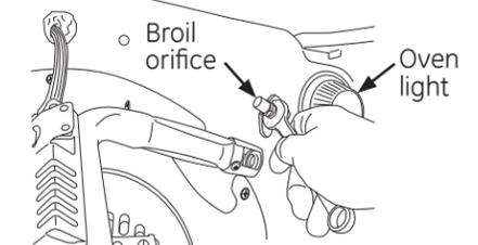
1. Remove the 1/4" hex screw securing the broil burner and allow it to hang down free of the broil orifice.
