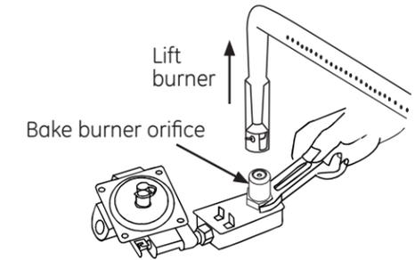
1. Remove oven racks, door, storage drawer and oven bottom. Remove the 1/4" hex screws securing the bake burner but don't remove burner from its location.
