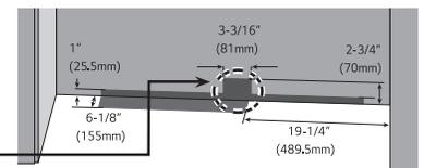
**Installation space for water supply pipe**
