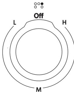
The control knobs can be set to anywhere between “H” and “L”. Push in and turn to setting.
