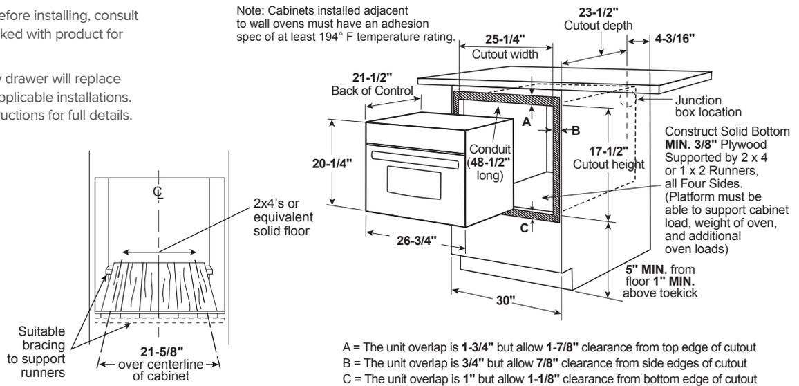
(Platform must be able to support cabinet load, weight of oven, and additional oven loads)
