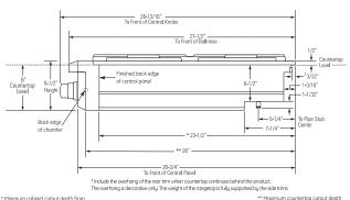
\* Minimum cabinet cutout depth from the back of the rear trinn to the back finished edge of the control panel tupically, the minimum cabinet depth [front to back] Maintum cabinet cutout depth is 26" minus the countertop \*\* Maximum countertop cutout depth from the back of the rear trim to the back edge of chamfer at the sides of the control panel - typically, the maximum countertop cutout depth front to back, Minimum countertop cutout depth is 25-1/4".
