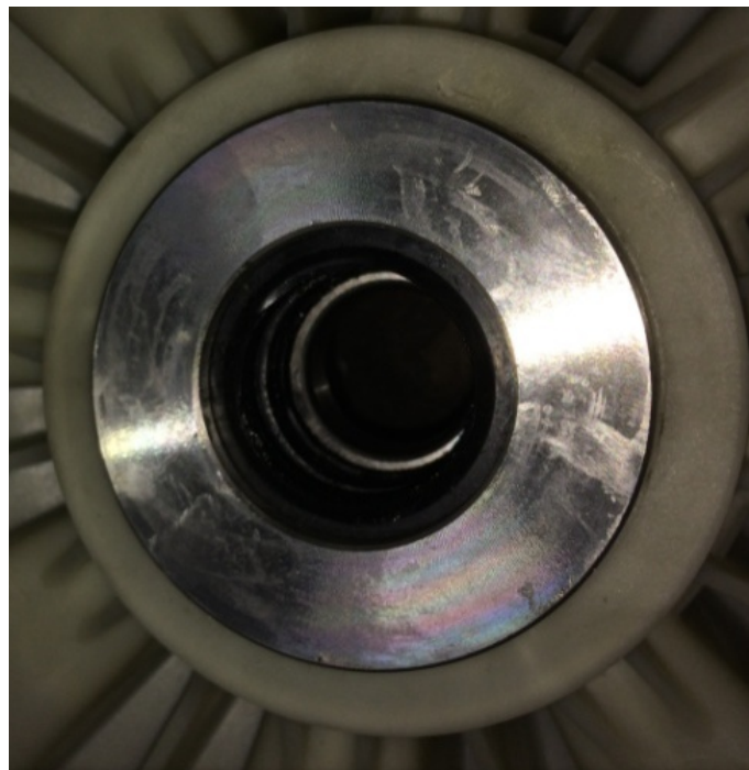
Figure 6. Water side Seal with 3.75" Washer (Item #2) covering.
