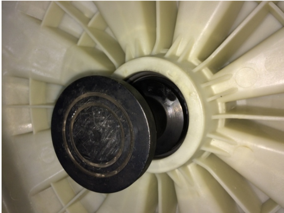
Figure 3: Use items #3 and #5 to seat the larger water-side bearing and smallest seal.
