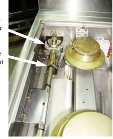
For the La Cornue ranges and hobs the regulator and the pressure tap can be found on the hob's manifold located by the 2 left gas burners
