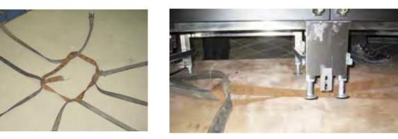
6. When lifting up stairs, the straps of the handlers at the bottom should be shorter so the cooker stays level.
