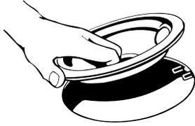
2. Holding the coil element as level as possible, slowly push the coil element terminal into the receptacle.
