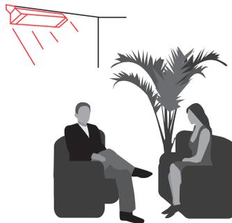
Install fixture to heat the area from the "cold side" if possible. This helps compensate for increased body heat losses due to exposure. Warm floors re-radiate heat. Warmer air rises from the floor. Some heat reflects from the floor. Mounting a heater directly over a table or other obstruction will block the energy, primarily heating the object. It is best to move heater to the side, allowing complete body and floor coverage.
