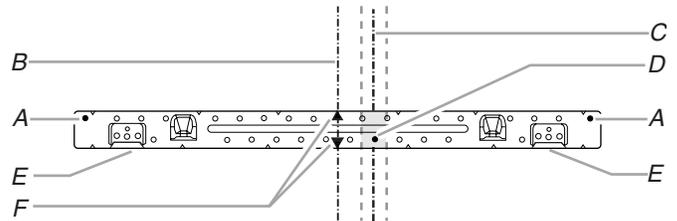
**NOTE:** If wall stud is within 6" (15.2 cm) of the vertical centerline (see "Mark Rear Wall" section), only recirculation or roof venting installation can be done.
