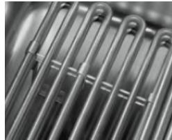
Internal electric resistance heater in the well with a rotating system for facilitating cleaning.
