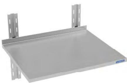
The shelf structure is made of 1 mm thick AISI 304 stainless steel and comes with a brushed finish. The double bent edges are rounded and welded to prevent dirt from building up and avoid sharp edges. This bracket mounted shelf has a rear upstand to prevent products from falling and can be adjusted to the correct height even after installation.
