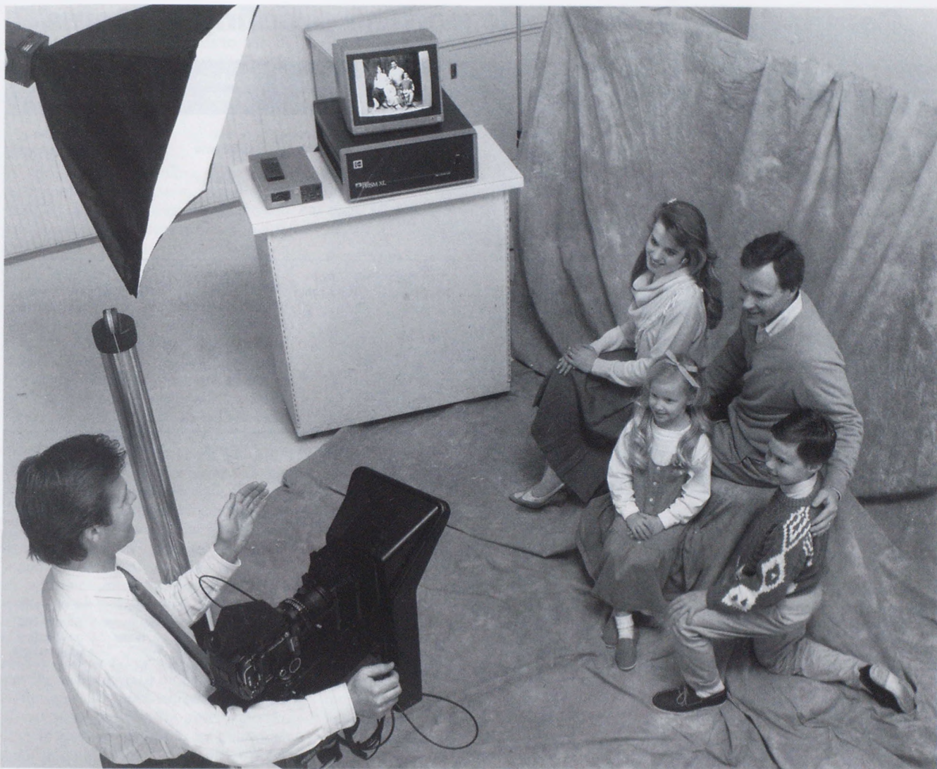
Kodak Prism XL is a fully-integrated electronic video proofing system designed for studio applications. The operator views a live video image displayed on the color television monitor—which matches that seen through the camera viewfinder. Still video images are recorded at the same time as studio camera flash exposures, so the photographer and subject can view sitting results and place orders before the photographic film is processed.
