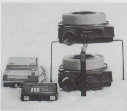
Audiovisual equipment required for a professional-quality civic or club slide presentation, as described by the author, includes two programmable slide projectors with two-tier stand, projector dissolve unit, with a two-channel or stereo tape player. In large halls, an amplifier and speakers may be added for better sound.
