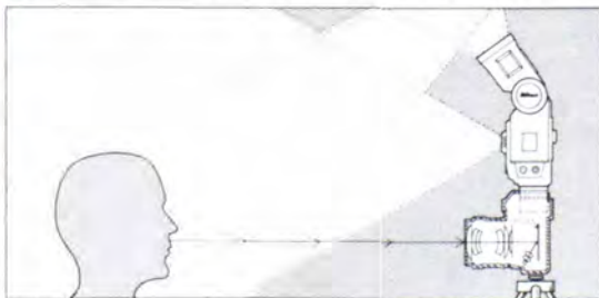
Nikon's automatic TTL metering system makes flash pictures as foolproof as existing light pictures.
