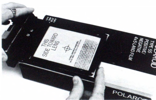
Cowan aligns film holder on box before making exposure. After he turns out the lights, he pulls the cover and places the holder back on box for proper exposure alignment.
