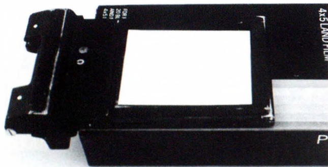
Cowan cuts white paper to fit inside film holder to focus slide prior to inserting and exposing film.
