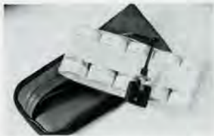
This external battery pack is set up to fit inside a Vivitar Pocket Instamatic case.
