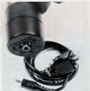
Here an RCA plug protrudes through a hole drilled in the bottom of a battery case cover.
