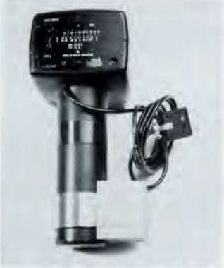
A hole drilled in a Rollei 140RES flash unit accepts a cord that leads to an external power pack.
