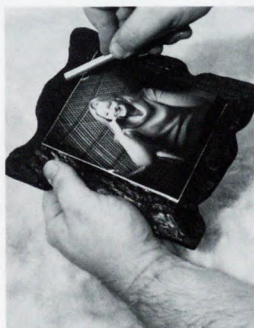
Outline the print with the handle of the X-Acto knife—this facilitates trimming. Note the plaque outline under the print at the bottom.
