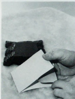
After peeling off the protective backing from the adhesive and exposing two inches of cold mounting material, align adhesive with print back, and apply.
