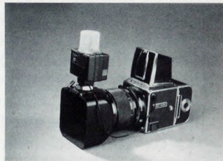
Converted bare-tube fill in place.
