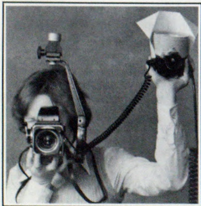
For round flash heads, the corners of the spill card should be bent back.
