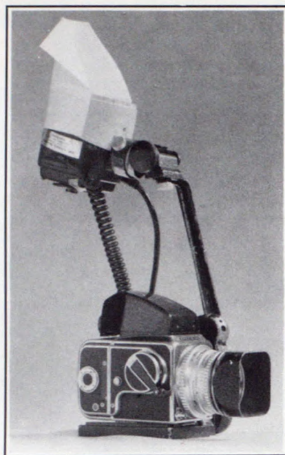
A closer view of a spill card in place on a round flash head.
