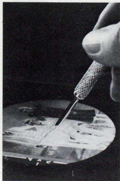
Right — Etching knife blade edge is parallel to negative surface.
