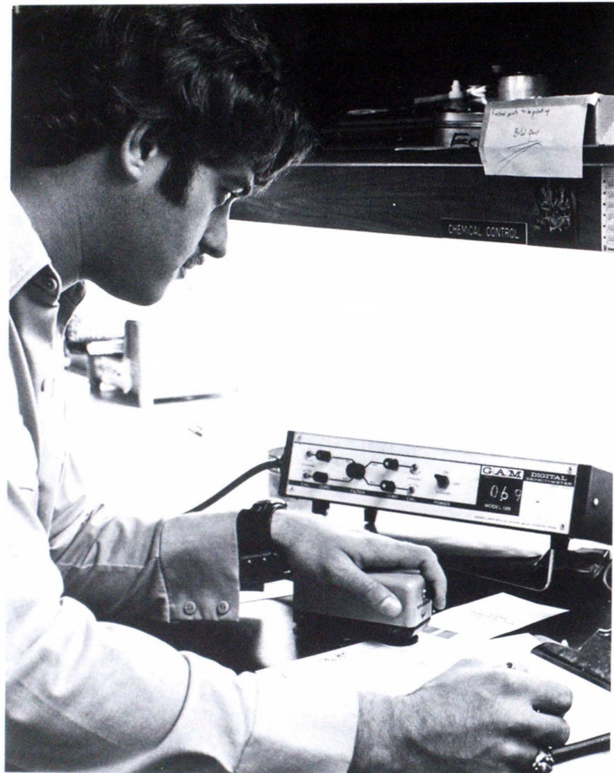
Studio prides itself on color control, using GAM Digital Densitometer. Chemicals are changed three times daily to maintain balance in portraits.
