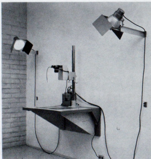
Copy stand, designed for making 35mm slides from flat copy, has proved useful with larger cameras.
