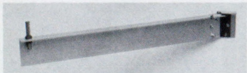
Above: Light bracket is of angle aluminum, swings on loose pin hinge. A 3/8" bolt, with head sawed off, holds lamp head. Right: Portion of hinge fastened to wall.
