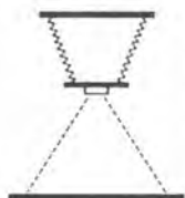
Negative stage, lens and baseboard locked in alignment.
