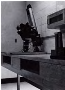
Dry side of color printing darkroom shows Chromega enlarger, anti-static device, and foot-candle meter.
