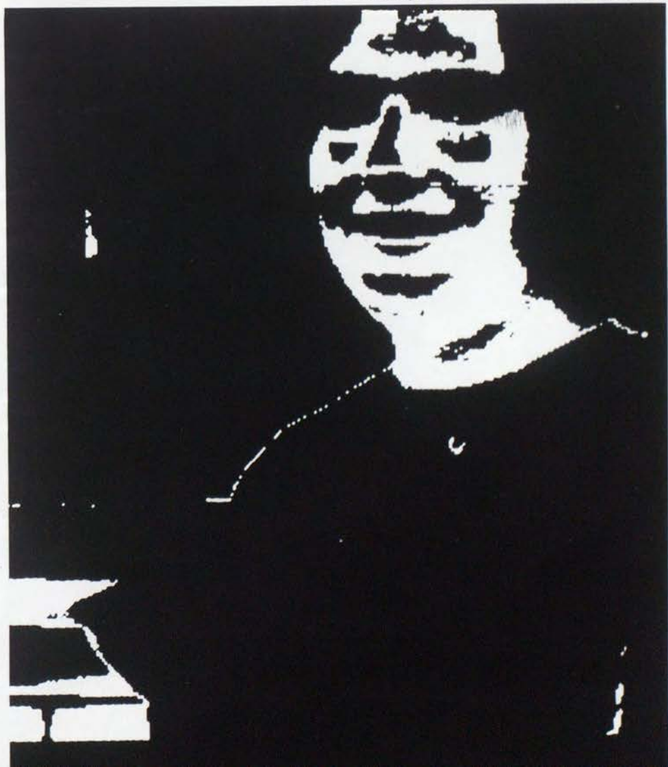
Computer-analyzed picture reducing continuous toned images to 8 component brightness levels. John Mott-Smith, Air Force Cambridge Research Laboratories, Bedford, Mass.
