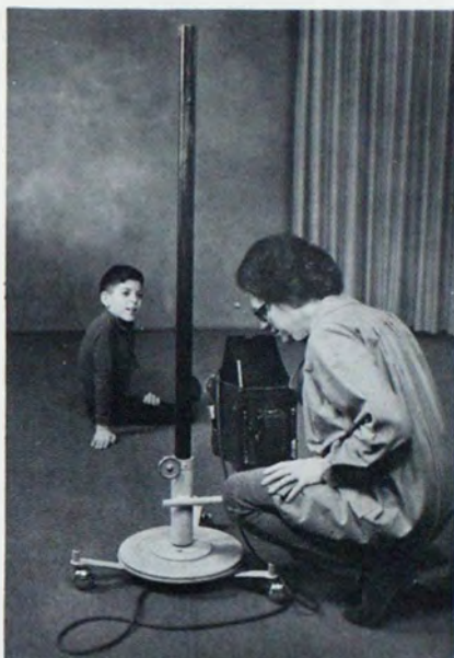
Camera is brought to almost floor level with home-made center post camera stand.
