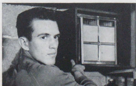
Below: Film safe of 3/4" plywood consists of one box which holds hanger rack and nests inside a second box mounted on the wall, forming a light-tight unit. Boxes were coated inside and out with black dulling lacquer. Safety was tested by flashing a speedlight outside and then developing film which had been stored inside. Right: Stoboflash head mounted on Crown Graphic using the Leica pan head provides flexibility of adjustment for the flash head and positive locking after positioning.
