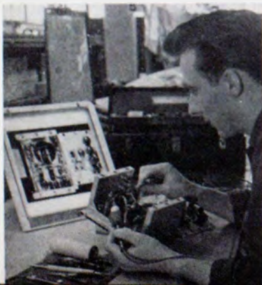
Above: Etched wiring patterns and switch parts made by photo-mechanical process at Hughes Aircraft Co. Below: Color transparency of wired prototypes serves as guide in wiring at Bell Aerosystems.
