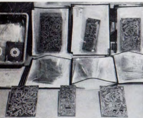
Above: Etched wiring patterns and switch parts made by photo-mechanical process at Hughes Aircraft Co. Below: Color transparency of wired prototypes serves as guide in wiring at Bell Aerosystems.
