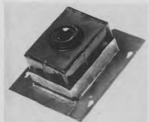
This illustration explains Mr. Bellah's set-back lens board as well as any diagram.
