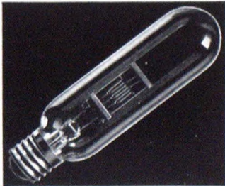
1000-watt T-20. Has a more concentrated filament than lamps in the PS-52 bulb. This helps provide better light concentration; permits crisper shadows.
