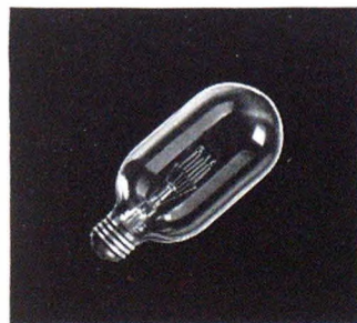
500-watt T-20. In clear glass. Often used in spotlights, because of its concentrated filament. Also available in inside-frosted photo blue.
