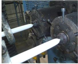
Representation of the extrusion die for manufacturing tubular profiles
