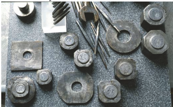
Figure 1 Original Dies & Tools used in the striking of Mormon Gold Coins
