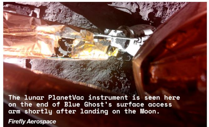
The lunar PlanetVac instrument is seen here on the end of Blue Ghost's surface access arm shortly after landing on the Moon.
