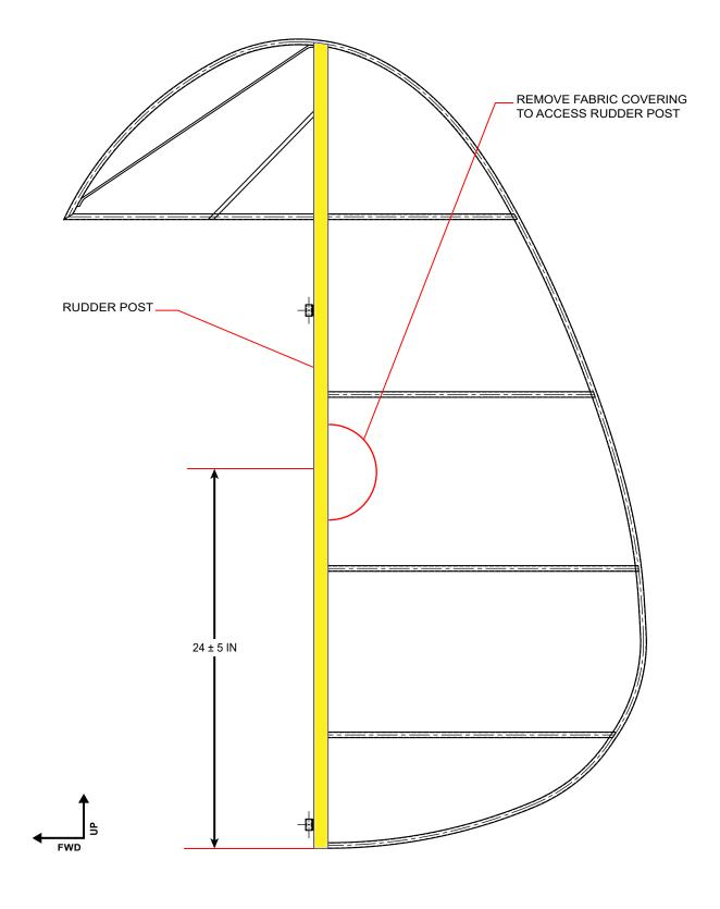
Figure 1 Rudder Assembly
