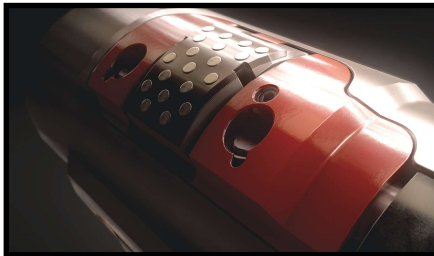
Weatherford’s Magnus RSS features fully independent control of three steering pads to selectively push the bit sideways. (Source: Weatherford)
