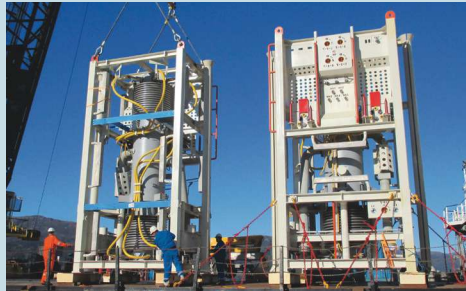
The world's first subsea multiphase compression system, which adds an estimated 22 MMboe, is shown being prepared for deployment. (Source: Schlumberger)
