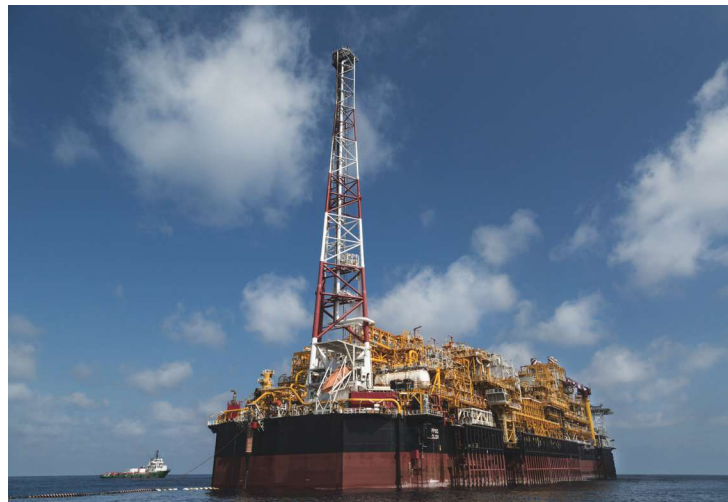
Total's Norte is Kaombo's first FPSO, which will produce about 115,000 bbl/d. (Source: ALP Marine Services for Total EP Angola Block 32)
