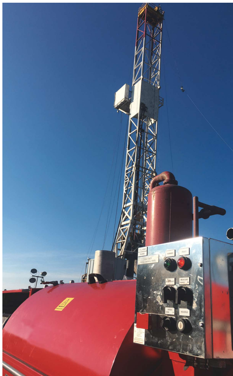
The MudCube is a compact, lightweight solids control system that can be added to existing operations. (Source: Cubility)
