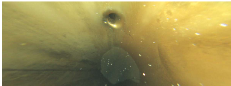
The Vision WellCAM produces high-resolution color images making perforation identification and measurement a quick and easy operation. (Source: Expro)
