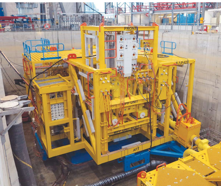
FIGURE 1. A high-viscosity, high-boost pump in a subsea pump station was tested at the OneSubsea test facility in Hørsø, Norway. (Source: Schlumberger)
