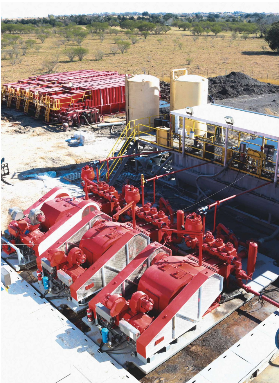
Three 1,600-hp, 7,500-psi mud pumps were added to Rig 16 as part of the upgrade. (Photo by Jennifer Presley)
