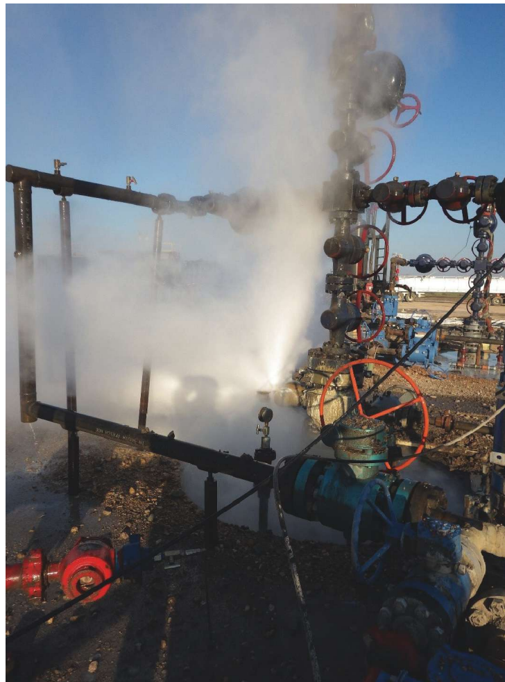
Wild Well responds to a blowout resulting from compromised wellhead equipment. (Source: Wild Well Control)
