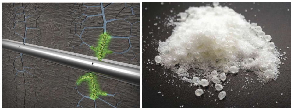
FIGURE 1a. Left, AccessAcid Stimulation service provides leak-off control properties at the fracture level by bridging off against the fracture face or formation face.
