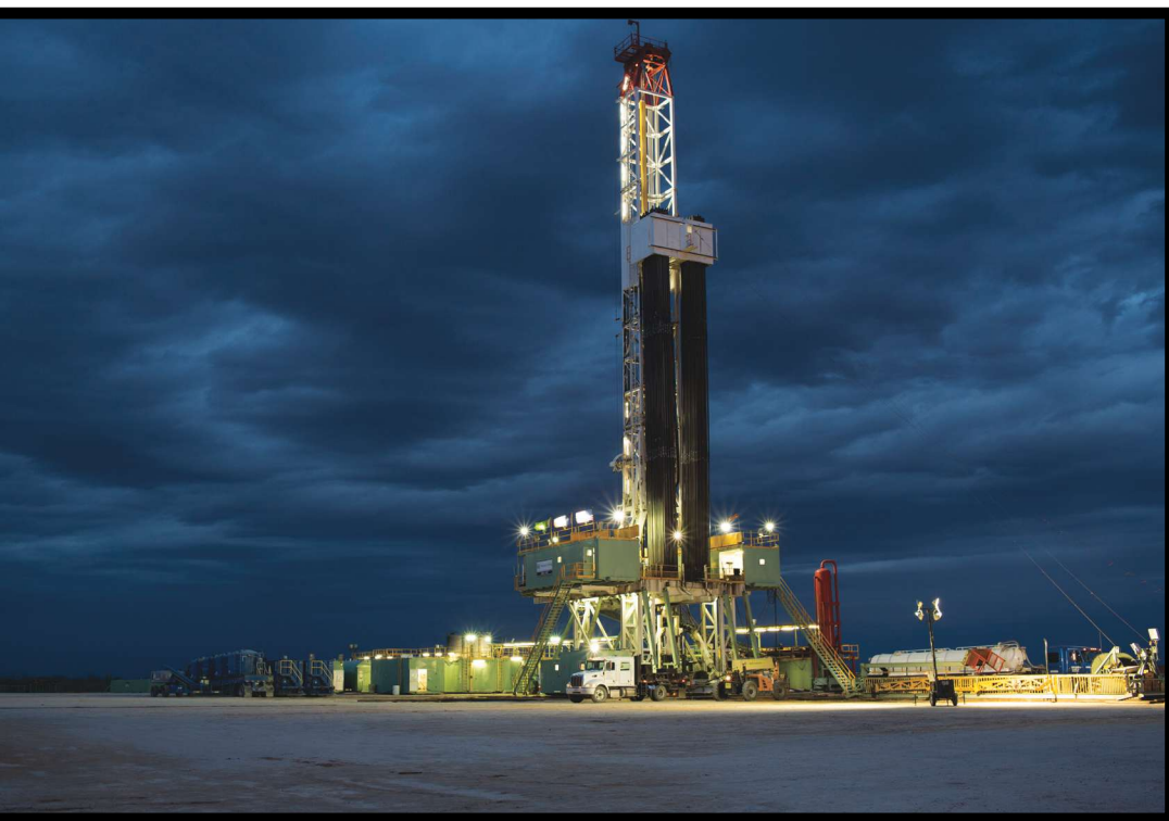
The Super Triple 1500 is equipped with full pad walking capabilities and high-pressure circulating systems. (Source: Precision Drilling)
