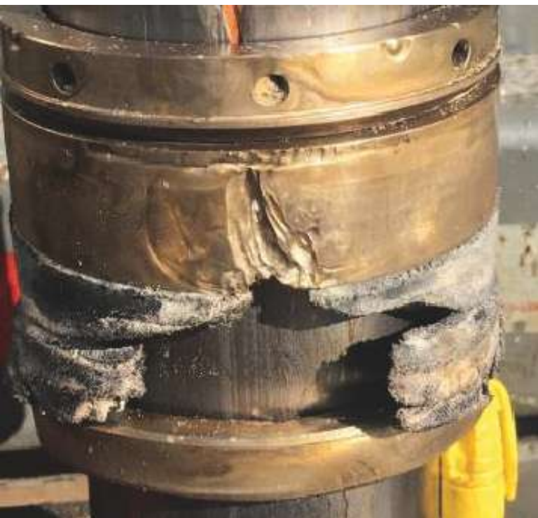
FIGURE 1. This image depicts catastrophic packing failure after 35 hours of operation. (Source: Gardner Denver)
