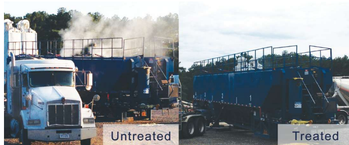
This side-by-side comparison shows airborne dust from untreated fracture sand versus the absence of dust from sand treated with SandTec. (Source: ArrMaz)
