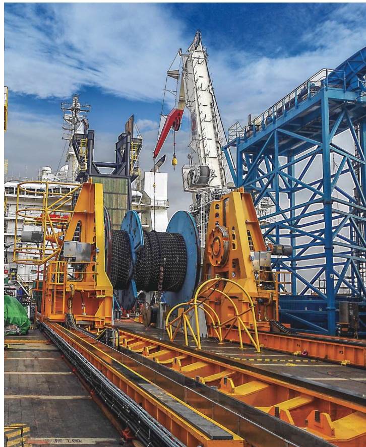
Reel drive systems deploy and recover umbilicals or flexible pipes that are stored on standard flexible product reels. (Source: NOV)
