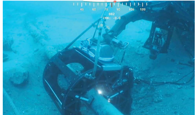
The Neptune ROV completed its deepest inspection to date in 2017 at 2,250 m water depth with equipment rated for 3,000-m buoyancy. (Source: Oceaneering)
