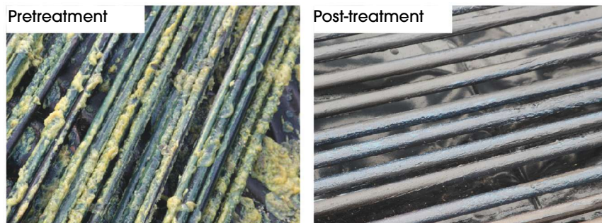
FIGURE 2. Sucker rods exhibit paraffin deposits when they are pulled before treatment, and no paraffin is present after treatment. (Source: Locus Bio-Energy Solutions)
