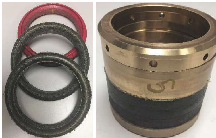
FIGURE 2. Redline Packing demonstrates no failures after 138 hours of operation. (Source: Gardner Denver)
