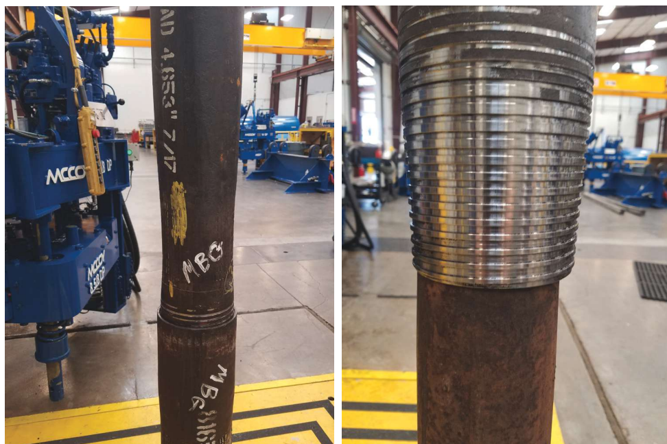
Left, during the application of high torque, the test subject 5.500 20.00# P110 pipe body was crushed at 46,500 ft-lb. Right, after the application of maximum torque, the TEC-LOCK Wedge connection was undamaged. (Source: Hunting Energy Services)
