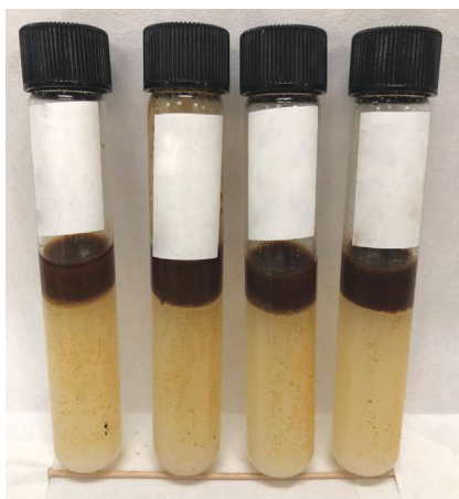
FIGURE 1. Liquefied paraffin dispersed within 25 minutes at 35 C (95 F) is compared to 20 minutes for toluene. (Source: Locus Bio-Energy Solutions)
