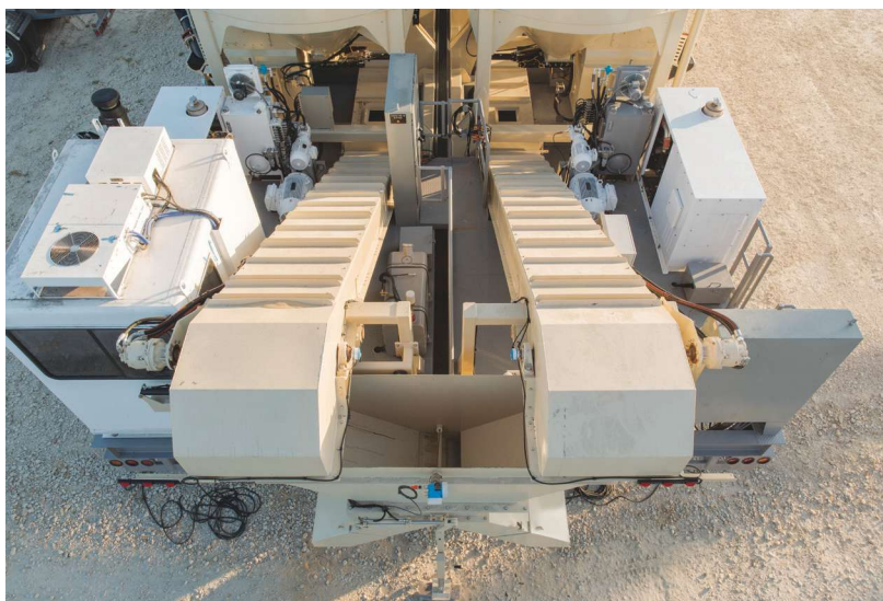
The SandBank loads a silo at 275 tons of proppant per hour using a bucket elevator system and feeds blenders between 700 lb/min and 20,000 lb/min of proppant using auto-controlled conveyors. (Source: NOV)
