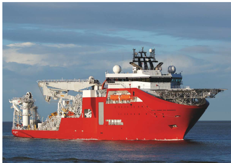
The Lewek Connector vessel is outfitted with a horizontal lay system. (Source: NOV)
