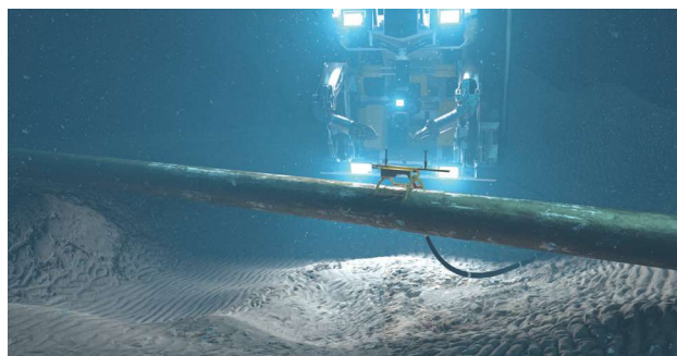
The Sea Turtle uses electromagnetic acoustic transducers to assess the plate or pipe condition of structures, pipelines, jumpers, flowlines and risers. (Source: Oceaneering)
