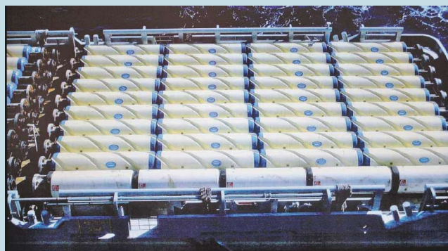
The Helically Grooved Buoyancy is deployed alongside the Ocean BlackRhino drillship. (Source: Diamond Offshore)
