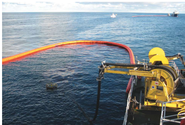
NorLense booms contain the spill and recover it onto a vessel with the Framo TransRec Oil Skimmer System. (Source: Framo AS)
