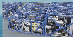
Skid Mounted Frac Pumps
