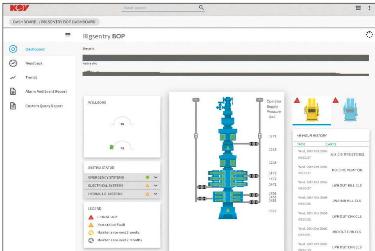
FIGURE 2. The Rigsentry BOP monitoring system provides critical equipment information in real time to predict failures. (Source: NOV)
