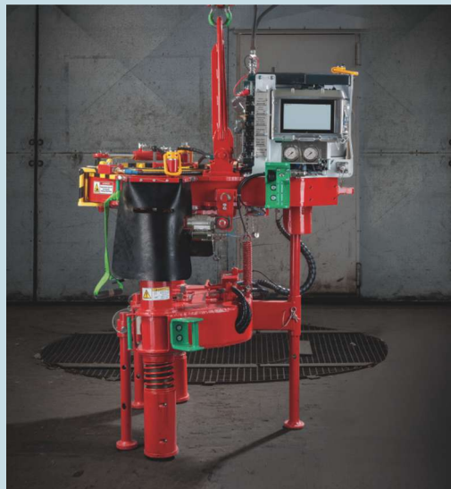
The AutoTong system delivers connection integrity with fewer personnel as it is operated by a single user for both the tong and torque-turns monitoring system. (Source: Weatherford)
