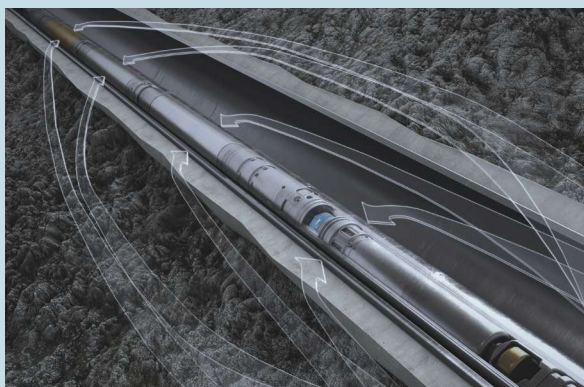
Pulsar multifunction spectroscopy service is a standalone cased-hole formation evaluation and reservoir monitoring service. (Source: Schlumberger)
