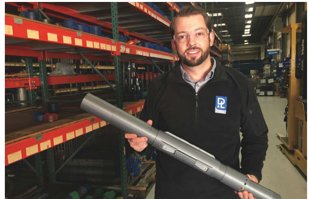
The Trilobite product name was inspired by the combination of "tri" for the three slips, "lob" for it being a lobe tool and "bite" for it being a way for things to bypass as well as the tool's literal bite, which keeps it in place, according to Heath Bringham (pictured), the original developer of the tool. (Source: D&L Oil Tools)
