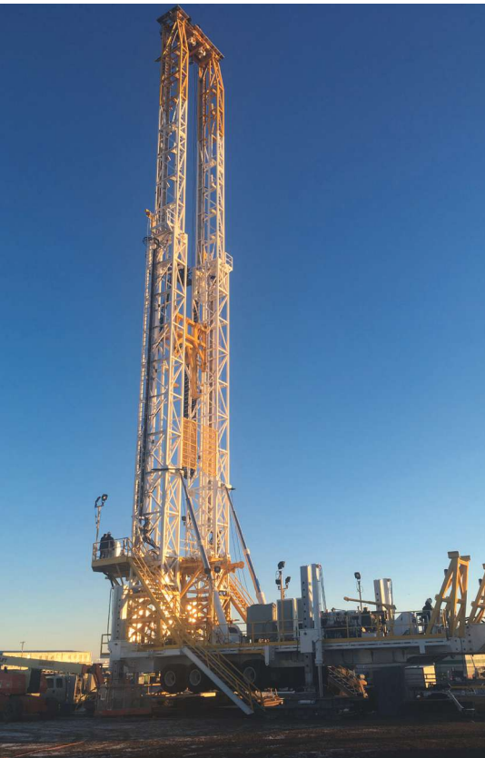
The XTD4 CTD rig is an all-electric fully connected integrated system. (Source: Schlumberger)
