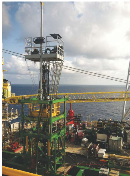
The CCTLF was used in four well completions offshore Nigeria. (Source: NOV)
