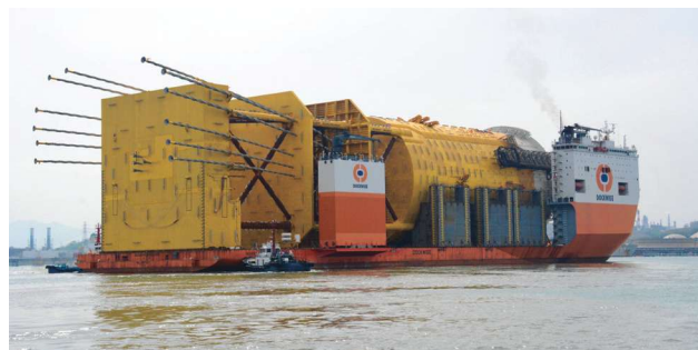
The Dockwise Vanguard transports the Aasta Hansteen spar from HHI in Ulsan, South Korea, to Ølensvåg, Norway. (Photo by Eva Sleire, courtesy of Statoil)
