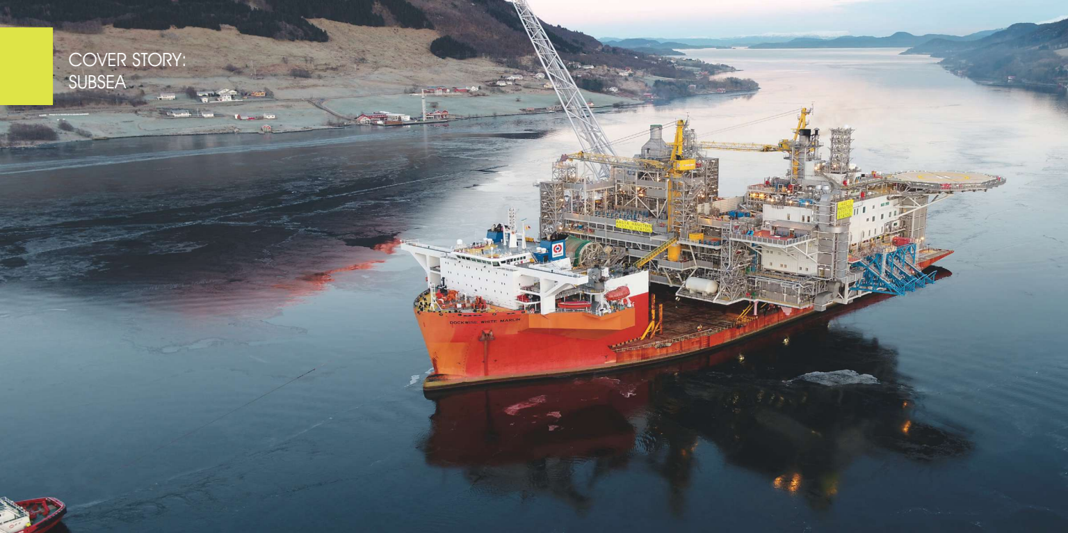
The heavy transport vessel Dockwise White Marlin transported the 24,000-tonne topsides for the future the Aasta Hansteen spar FPSO unit from the Hyundai Heavy Industries' shipyard in Ulsan, South Korea, to Ølsvåg, Norway, in late 2017. (Photo by Espen Rønnevik/Worldcam, courtesy of Statoil)
