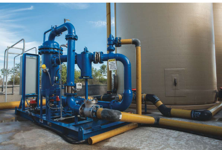
The Tore Trap skid from NOV desands up to 18,000 bbl/d. (Source: NOV)
