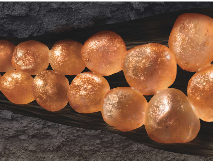
FIGURE 1. Hexion's OilPlus proppants increase the relative permeability of oil in the proppant pack. (Source: Hexion Inc.)
