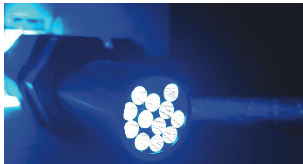
Optical waveguides glow as they transfer light into the reactor's shell. (Source: Cornell University)
