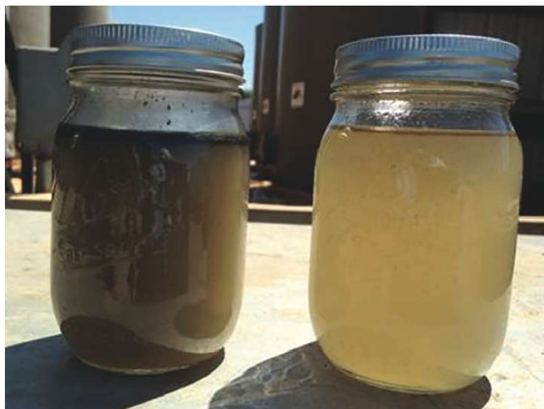
Pictured are a water inlet sample to the Tore Trap (left) and a desanded water outlet sample (right). (Source: NOV)
