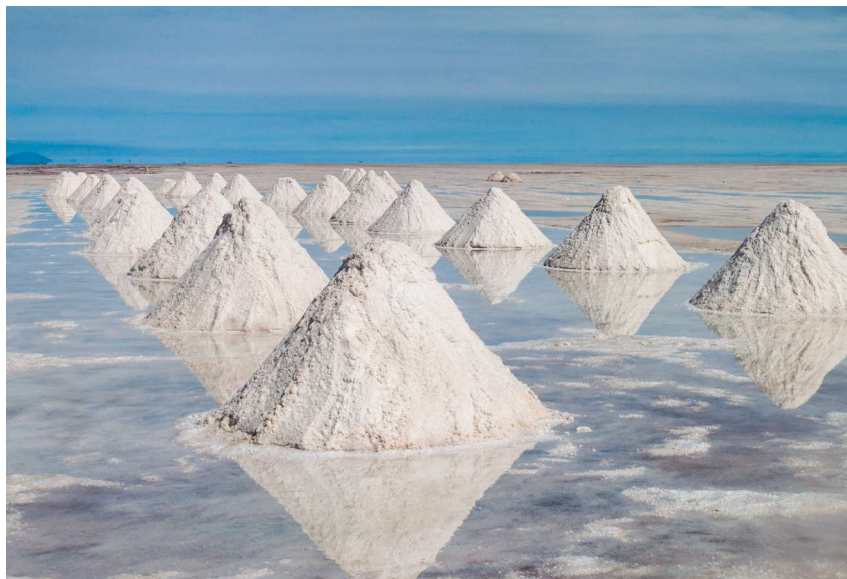
Hand-shoveled salt piles dry on Bolivia's Salar de Uyuni, thought to be one of the richest sources of lithium in the world. Solar evaporation takes up to 18 months. (Source: Matyas Rehak, Shutterstock.com)
