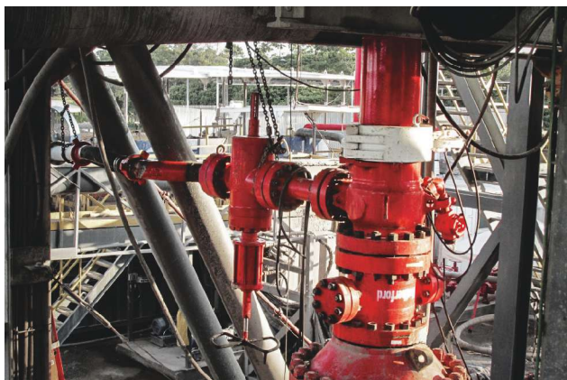
The SafeShield RCD enables MPD techniques in a wide range of applications, including high-pressure wells. (Source: Weatherford)
