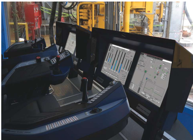
Integrating MPD controls into the driller's interface enables reductions in NPT by putting the driller in control of the MPD process. (Source: NOV)
