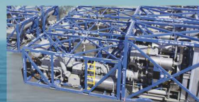
Skid Mounted Frac Pumps
