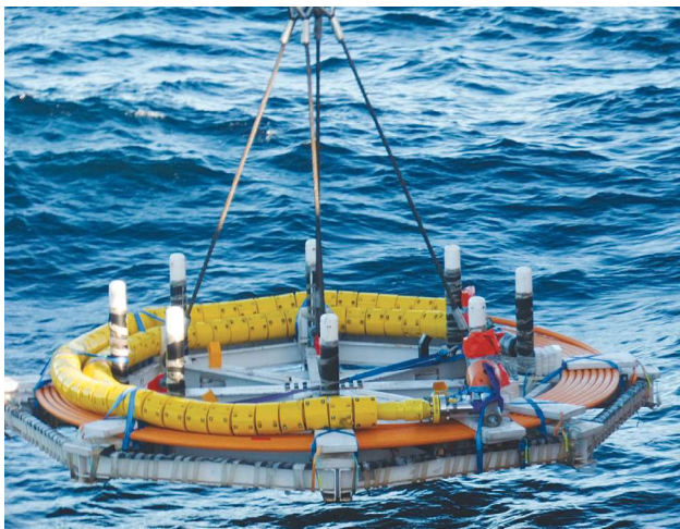
An HP/HT composite jumper is being supplied for the Alder Field developments. (Source: Airborne Oil & Gas and Chevron North Sea Ltd.)
